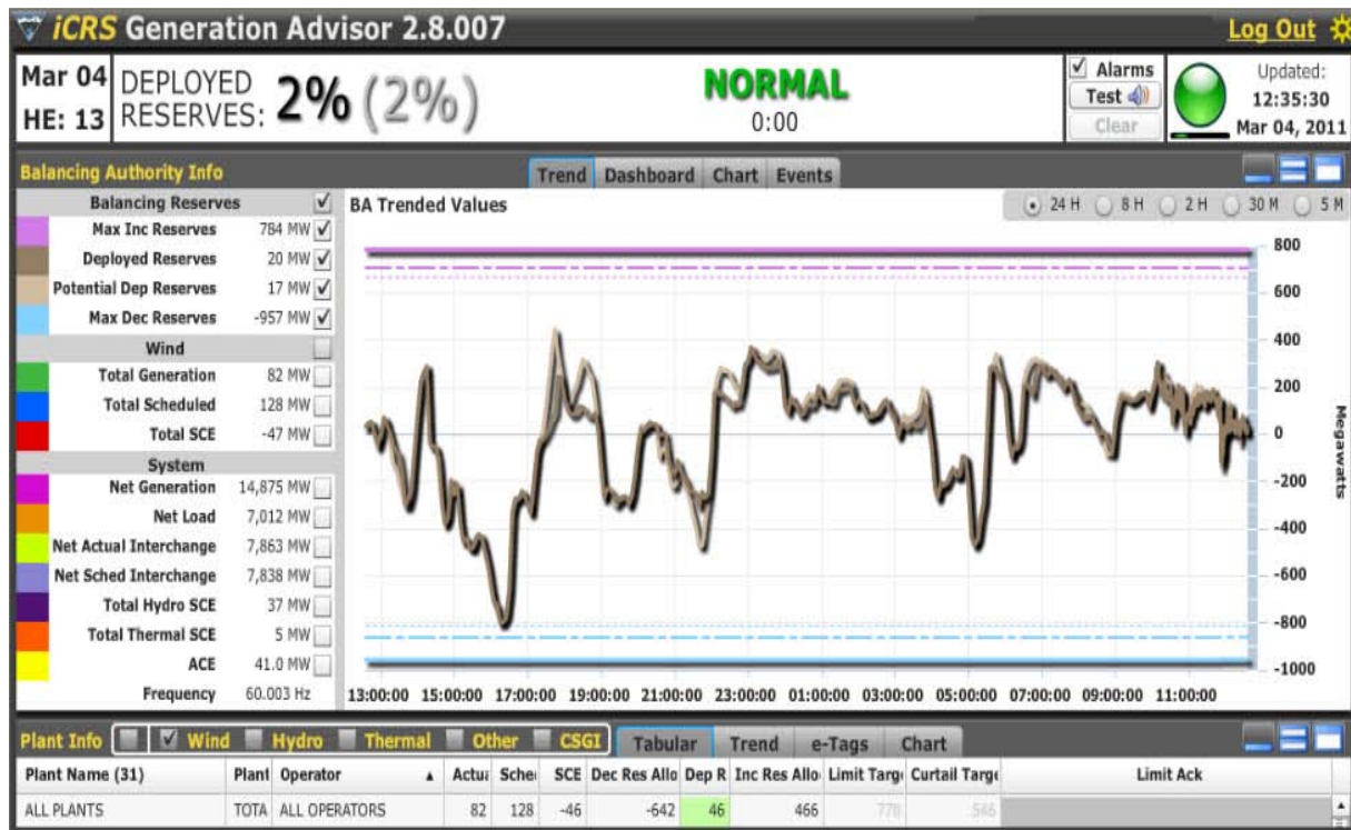
Figure 60. iCRS Generator Advisor Trend Display of Balancing Reserves (Provided by Bart McManus, BPA)
