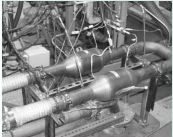
NO<sub>x</sub> adsorber catalysts were installed in this test cell at FEV in Auburn Hills, MI.
