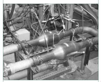
$\mathrm{NO}_{\mathrm{x}}$  adsorber catalysts were installed in this test cell at FEV in Auburn Hills, MI.
