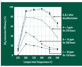
Figure 9. Comparison of NO<sub>x</sub> conversion efficiency before and after desulfurization for catalysts aged as long as 250 hours with 3-, 16-, and 30-ppm sulfur level fuels
