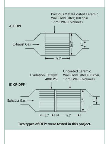
engine (which has a relatively low temperature exhaust) was tested using the OICA 13-mode test procedure and tests at peak-torque and "road-load" steady-state conditions. Regeneration temperatures were determined at selected engine speeds by measuring the change in pressure across the DPFs while operating the engine at different temperature and torque settings.
