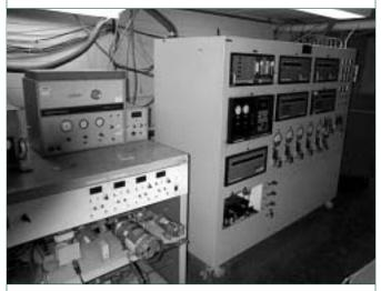
Emissions benches like this one at WVU were used to collect data during the tests.
