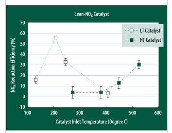
Figure 2. NO<sub>X</sub> reduction efficiency of low-temperature (Navistar) and high-temperature (Cummins) lean-NO<sub>X</sub> catalysts at selected catalyst inlet temperatures (with 95% confidence intervals)
