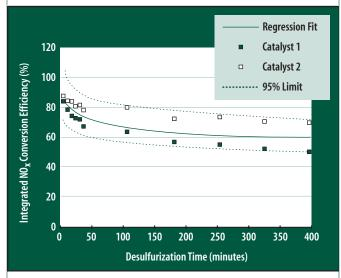
Figure 10. Regression model (with 95% confidence interval) of post-desulfurization NO<sub>x</sub> conversion efficiency versus total desulfurization time. Data for catalyst pair aged on 78-ppm sulfur level fuel.
