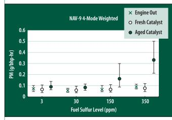
Figure 4. Engine-out and fresh, aged lean-NO<sub>x</sub> emissions of PM under low-temperature (Navistar) applications using the Nav-9 weighted 4-mode test cycle (with 95% confidence intervals)
