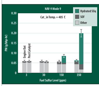
Figure 5. Engine-out and post-DOC (fresh) emissions of total PM and components under low-temperature (Navistar) applications using a Nav-9 mode 9 test (with 95% confidence intervals on estimated PM)
