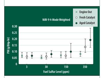
Figure 7. Engine-out and fresh, aged DOC emissions of PM under low-temperature (Navistar) applications using the Nav-9 weighted 4-mode test cycle (with 95% confidence intervals)
