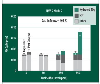
Figure 3. Engine-out and post-lean-NO<sub>x</sub> catalyst (fresh) emissions of PM and components under low-temperature (Navistar) applications using a Nav-9 mode 9 test (with 95% confidence intervals on estimated PM)
