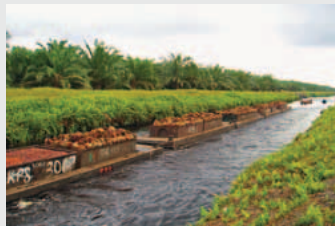
FIGURE 35 Water transport system for fresh fruit bunches to the palm oil mill using pontoons.
