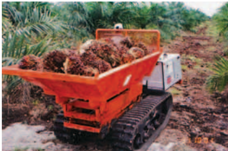
FIGURE 4 3 Tracked machine on soft ground.
