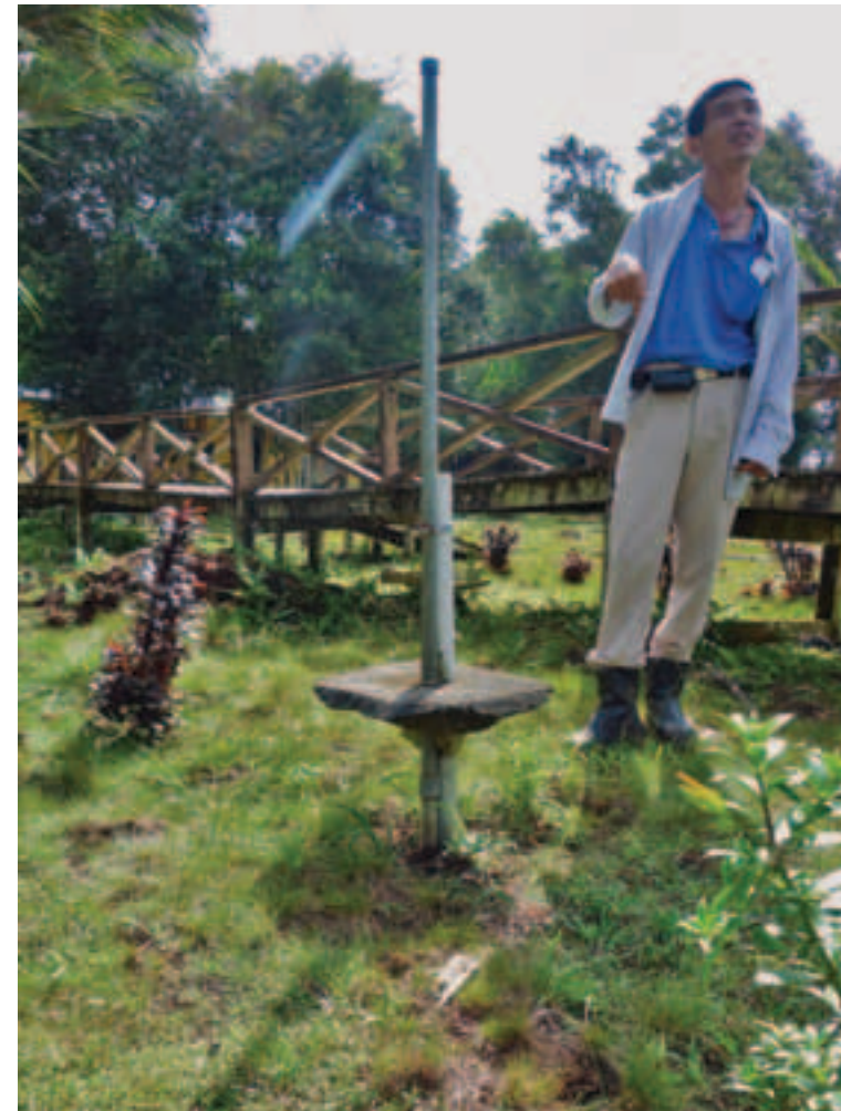
FIGURE 3 Example of subsidence pole installed together with a piezometer. Peat subsidence over time in this site is clearly visible.
