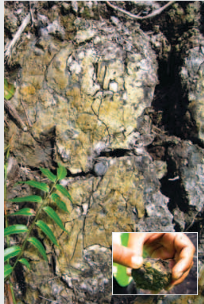
FIGURE 29 Acid sulphate soils. INSET Pointing out trademark yellow markings of acid sulphate soils.
