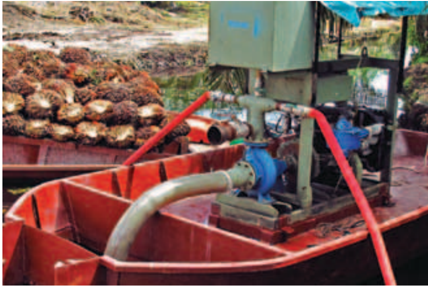
FIGURE 5 2 Close up example of fire boat used for fire suppression activities in oil palm plantations on peatland.
