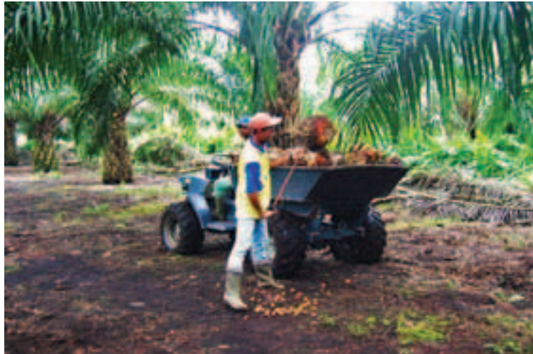
FIGURE 4 2 Low ground pressure (LGP) tyres on compacted path.
