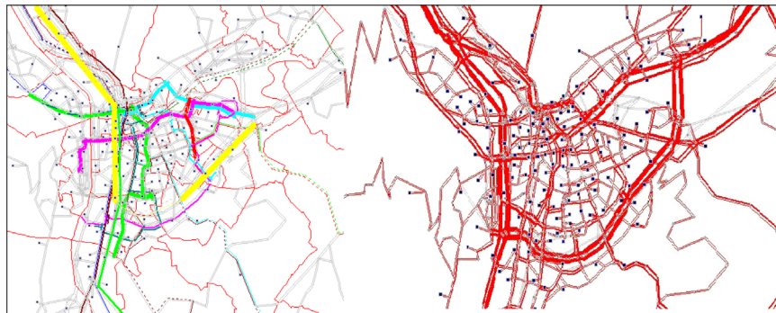
Fig. 7. the transport network in TRANUS, on the left the tramway lines, where each point is a zone of the model (where jobs and household by types are described); on the left the road network with a width proportional to capacity (authors).
