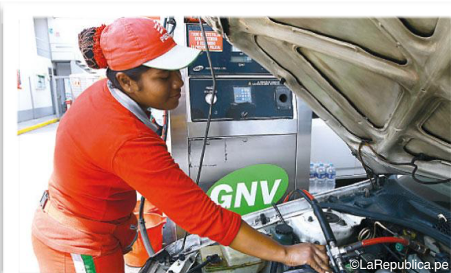
If the CNG (GNV) pump does not recognize the vehicle's ICT “smart charging” chip, the hose will not unlock.
