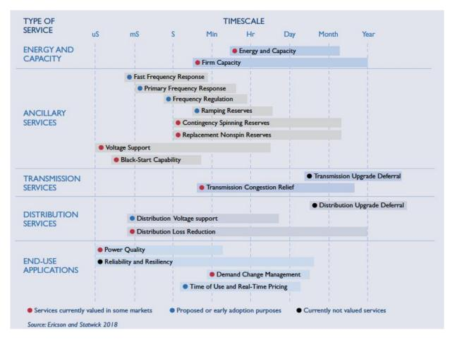
Figure 4: Timescale over which different battery storage services are provided Source : USAID 2020, https://pdf.usaid.gov/pdf\_docs/PA00X4KB.pdf
