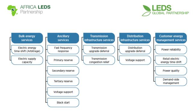
Figure 3: Functions of battery storage
