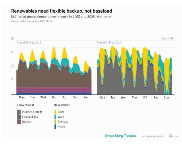
Figure 2: Illustration of Power Demand Patterns in Germany 2012 and 2020
