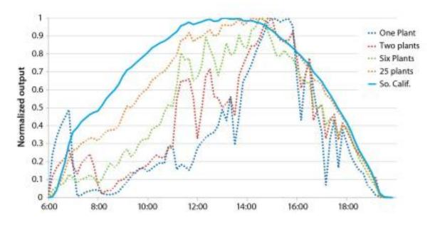
Figure 1: Output profile of different solar PV projects, including in all of Southern California
